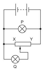
The slider on the potential divider is moved from end X to end Y of the resistor.
