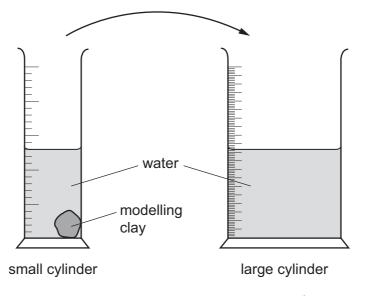
The reading on the small measuring cylinder goes down by 20 cm<sup>3</sup>.
