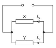
$I_X$  is the current in resistor X.  $I_Y$  is the current in resistor Y.
