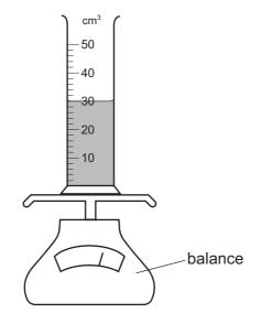
Some more of the liquid is added until the liquid level reaches the 50 cm<sup>3</sup> mark.
